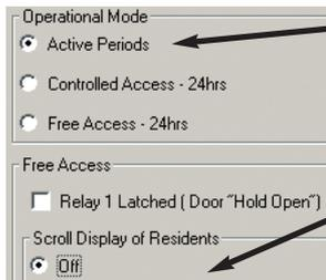
During an **Active Period** ie whilst the panel is displaying **FREE ACCESS** with an → arrow pointing to the ☎ button on the panel, the ⬆⬆ arrows used to scroll the display to find a particular Resident are totally disabled. The Scroll Display is not available. Pressing the ☎ button opens the door.
