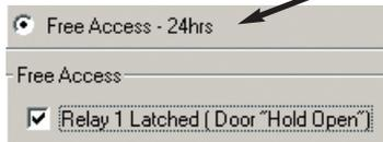
With **Free Access – 24hrs** and **Door “Hold Open”** selected, the panel also displays **FREE ACCESS** with an → arrow pointing to the ☎ button on the panel. The door is, however, in an UNLOCKED state 24 hours a day, so there is no need to press the ☎ button. This feature is mainly used on Visitor Days, Refurbishments, Furniture Removals / Deliveries etc.
